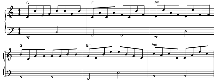
Fig. 4. An encoding of a 96-bit packet “36FB 224D 3935 C55F 4BE4 981E” using the baroque theme. (The top staff represents the data.)
