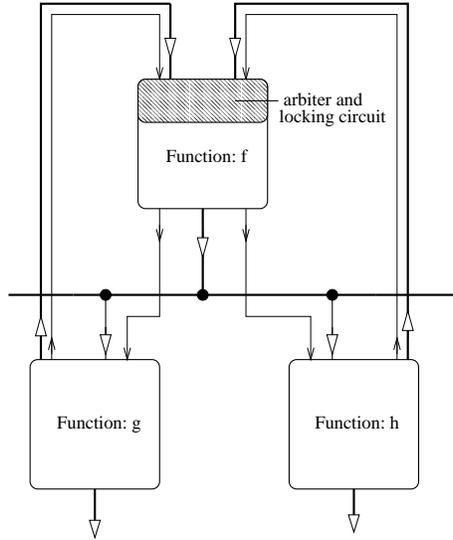
**Fig. 3.** A structural diagram of the hardware circuit corresponding to a shared function,  $f$ , called by functions  $g$  and  $h$ . Data buses are shown as thick lines, control wires as thin lines.
