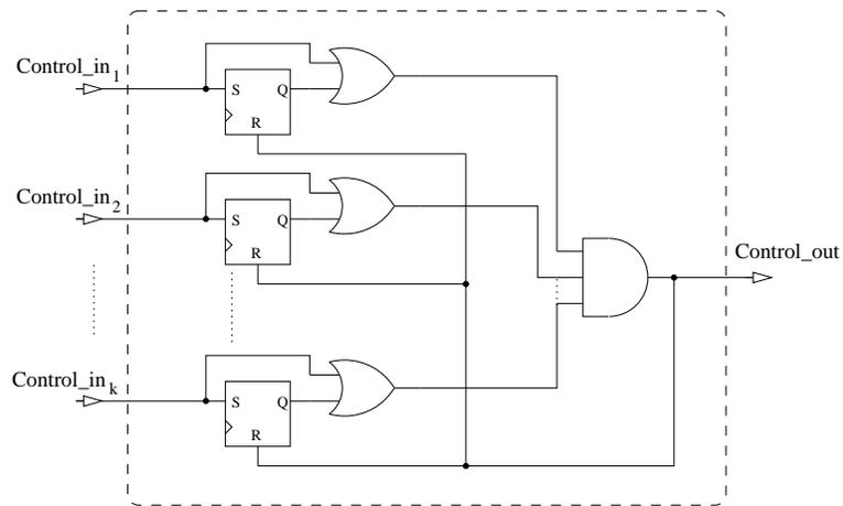
Figure 15: Hardware block corresponding to a CONTROL\_JOIN node
