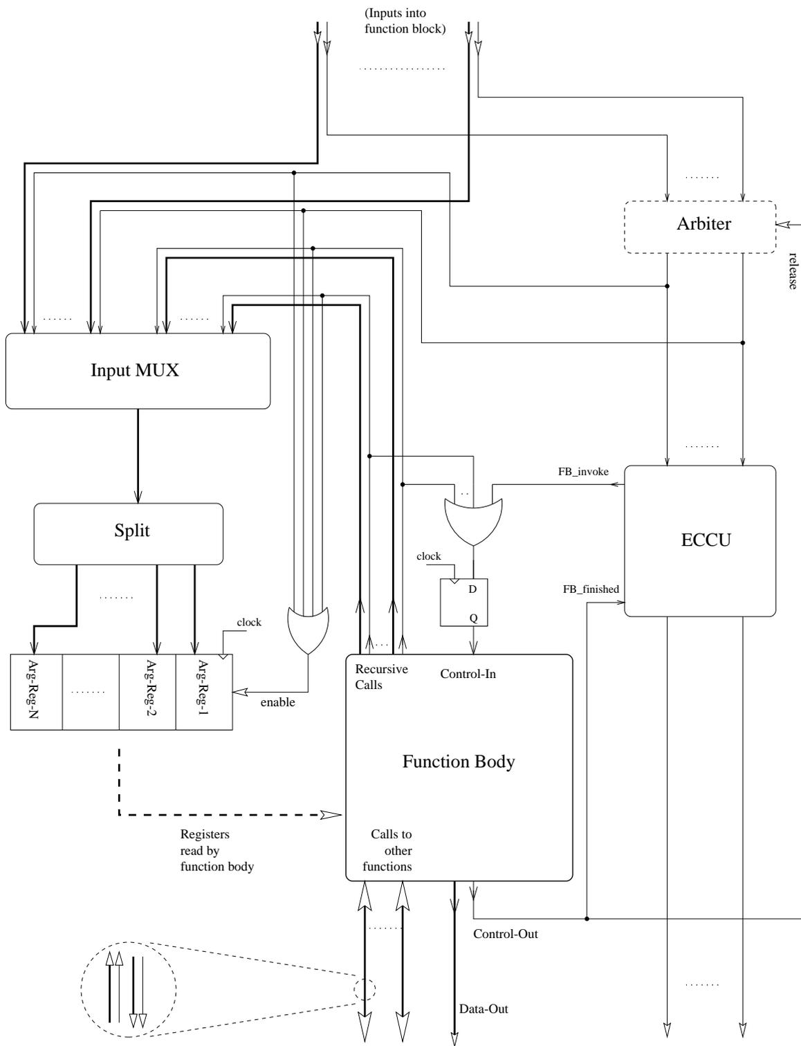
Figure 17: A Block Diagram of a Hardware Functional-Unit
